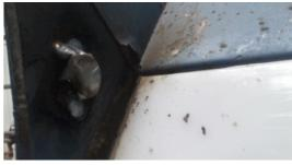
9. Reinstall the auger shield. The angle brackets that hold the shield in place on the from of the car will need to be loosened and slid up to allow for the thickness of the liner.
