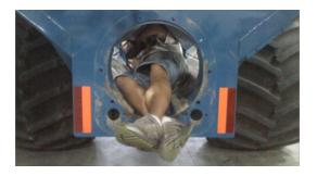
Once the auger is removed, the shield over the auger has to be removed. We recommend doing this by crawling into the cart through the back. If you are unable to do this remove the upper wire mesh grates to access the shield. The shield is bolted to the floor of the cart as well as to the front of the cart. Also remove the 4 bolts that splice the shield together in the middle.
