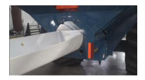
4. Slide the notched liner into the cart through the rear opening. Insert the notched end first. Slide the liner all the way forward until the notches hit the front auger housing.
